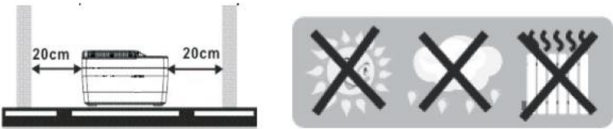
Figure 1. Placing of the UPS
